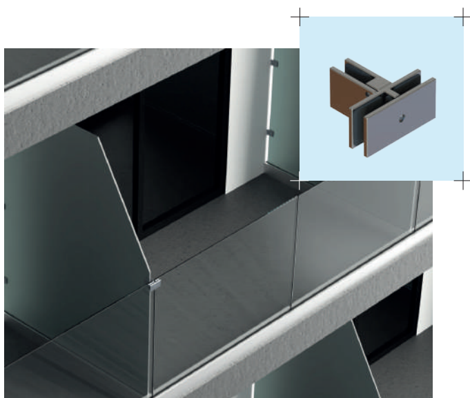
GLASS BALCONY PARTITION WITH RAILING SYSTEM AND SIDE CLAMP and connection solution to the guardrail in between glazings
