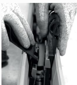
The complete tool is used to put the wedges in the rail.
